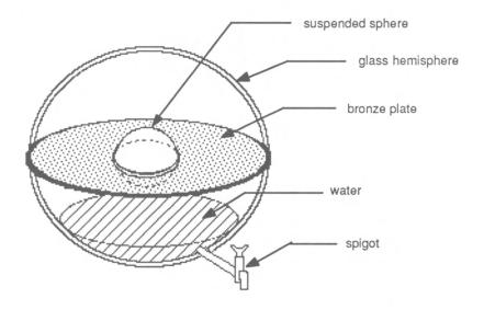
Figure 2. Teaching aid designed by Hero to show how stationary air could support a sphere
