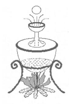
Figure 1. Hero's teaching aid for demonstrating the power of pneuma
